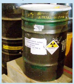
Can you easily find at least 2 issues with this shipment? Specifically, look at the two drums and the proper shipping name marking for surface contaminated objects. Should it be "Radioactive material, surface contaminated object" or Radioactive Material, SCO"?
