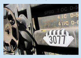
Cannot find enough flat-surface on your conveyance or package to apply your placard correctly? Are we allowed to wrap the placard around components like this on our rail cars or vehicles? Will anyone notice the hazard class is not in plain sight?
